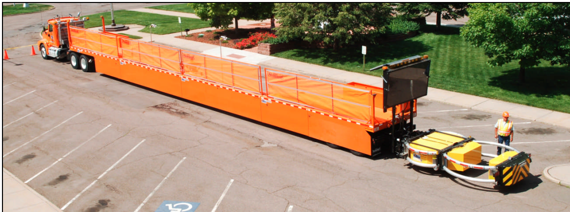
The Mobile Barrier Trailer MBT-1. Note the integral screens, TMA and illuminated arrow board.
