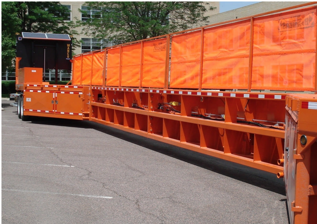
View from the works side of the mobile barrier trailer with screens installed
