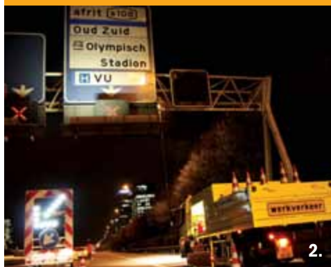
1. US firm Mobile Barriers recently won the International Road Federation (IRF) 2012 Innovative Product Award for its MBT-1 barrier for temporary highway work zones 2. M.A.R.S vehicle from TrafiQ is improving highway work zone safety on a number of Dutch managed motorways 3. Lafarge Tarmac's (UK) National Contracting division has introduced innovative technology offering greater protection for lone highway workers
